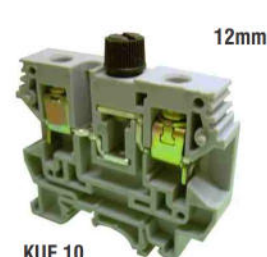
KUF 10 1000V/12A/10sq mm/1.4Nm
