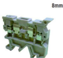
KUDF 4/D 800V/6.3A/2.5sq mm/0.4Nm
