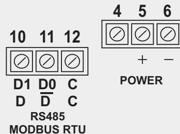
Obs.: Terminals 6 and 12 are connected internally.
