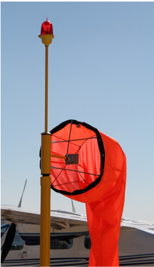
Orange Windsock attached to Red Obstruction Light
