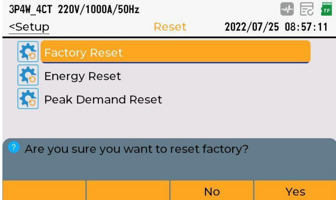
Figure 5- 32 Operation confirmation interface
