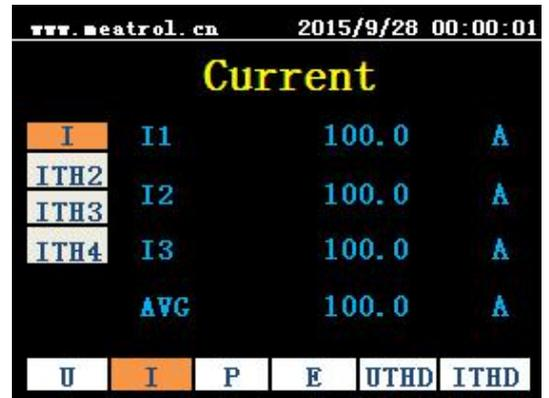
The secondary menus, from top to bottom are: I (current), ITH2 (2 harmonics current), ITH3 (3 harmonics current), ITH4 (4 harmonics current).
