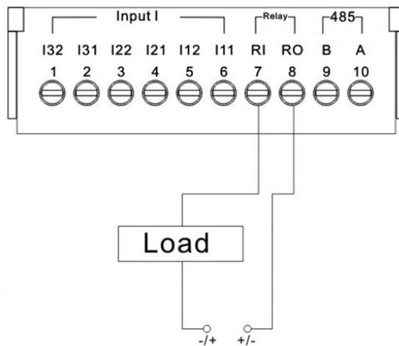
**Input&output Wiring diagram**
