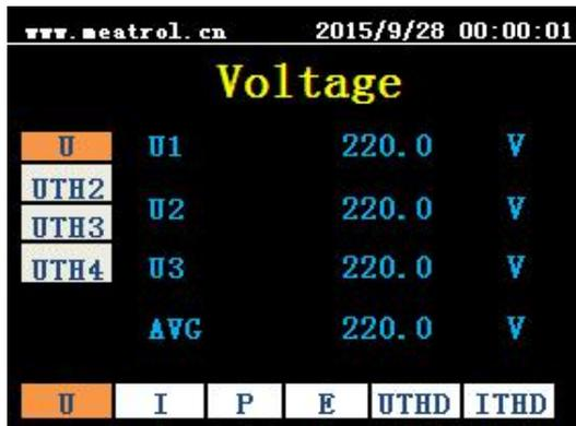
The secondary menus, from top to bottom are: U (voltage), UTH2 (2 harmonics voltage), UTH3 (3 harmonics voltage), UTH4 (4 harmonics voltage).
