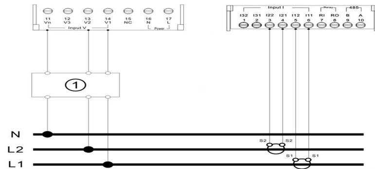
**ModBus communication Wiring diagram**
