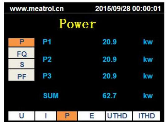
The secondary menus, from top to bottom are: P (active power), FQ (reactive power), S (apparent power), PF (power factor).
